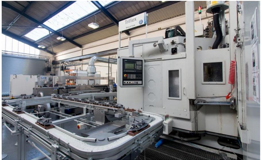
precision engineering operations, such as complex machining, cleaning and pressure testing of volume aluminium die castings.
